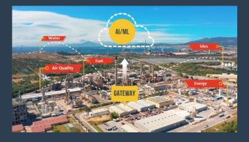
We have built all our hardware and software based on LoRaWAN technology. LoRaWAN is an globally accepted open source network which was developed by companies like Intel, Cisco etc. The Gateway when installed gives a wireless private network of about 1-1.5 km. All the assets within this range, can be push the data wirelessly to the Gateway.
